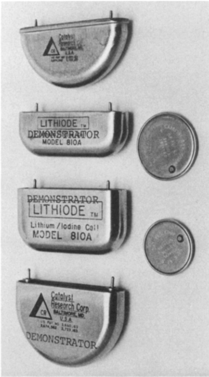
Fig. 1. Some pacemaker and button lithium-iodine cells. Large button cell is 23 mm in diameter.
